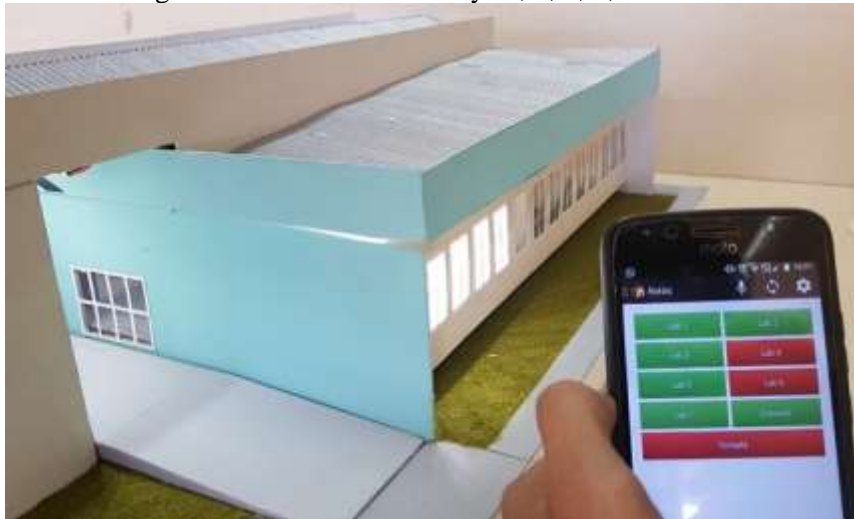
Figure 3 - Activation of Relays 1, 2, 3, 5, 7 and hall
