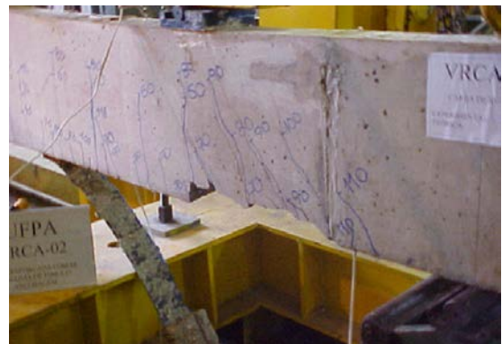
Figure 1 – Concrete cover detachment in a CFRP strengthened beam (ROCHA, 2013)
