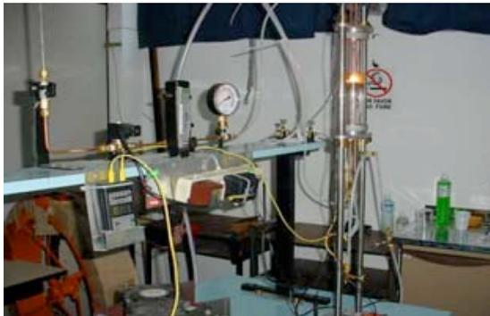
Fig. 1 – Hot Filament Reactor setup
