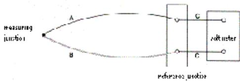
Figure 1 Simplified schematics of a thermocouple.
